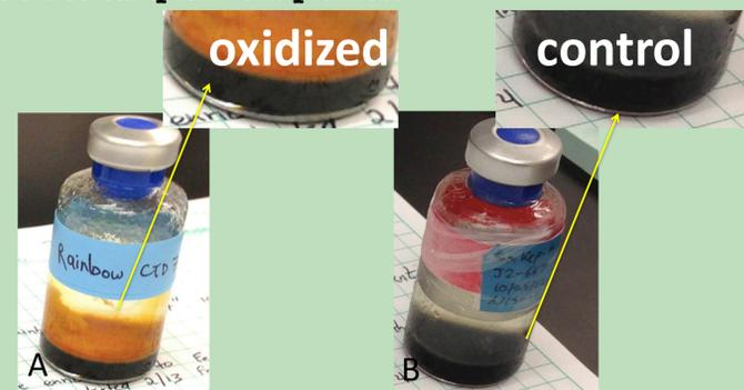
**Figure 3: A positive growth bottle indicated by a defined oxidation of the iron-sulfide agar plug (A) as compared to an uninoculated or negative growth bottle (B).**
