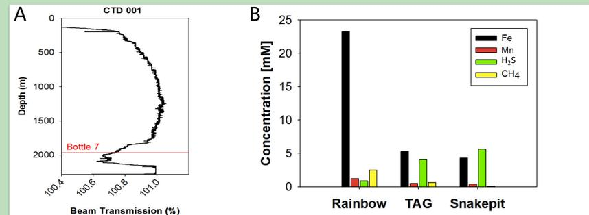
**Figure 2: A) Location of Niskin bottle deployment within the plume as indicated by transmissivity data. B) Concentration of various ions across the three sampled vent plumes.**
